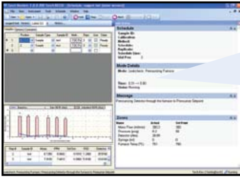
Leak Check Screen - The Leak Check screen identifies the region of the system that is being checked and the time remaining of the leak check.
